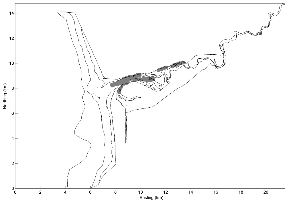
Figure 5.8 – Locations of measured bed forms extracted from the side scan sonar data set in the Dyfi. Dark grey areas represent the coverage of bed form measurements.
