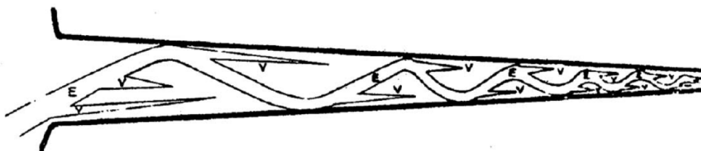
Figure 2.7 – Schematic representation of a Dutch tidal basin, highlighting flood- and ebb-dominant channels in the network (‘V’ and ‘E’ on the figure, respectively). From Van Veen et al. (2005)
