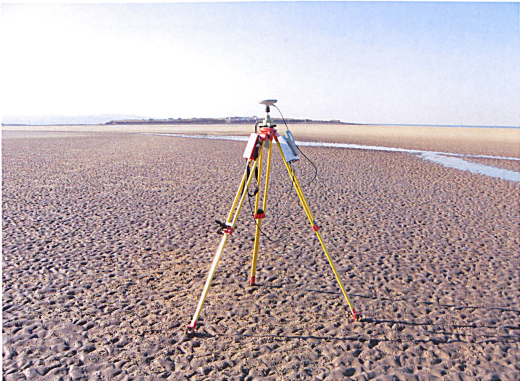
Figure 3.10: The DGPS base station set up on West Kirby Sands for the intertidal beach survey.
