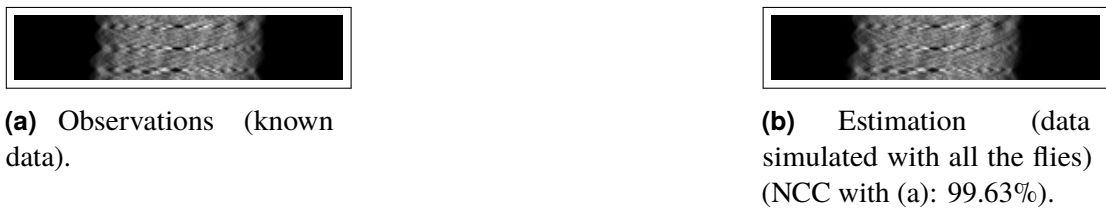
Figure 5.19: Sinograms from Figure 5.20a corresponding to the hot rod phantom with a low resolution and with noise. Images with 185 pixels per projection, 1 st angle: 0°, angular step: 5°, and last angle: 175°.
