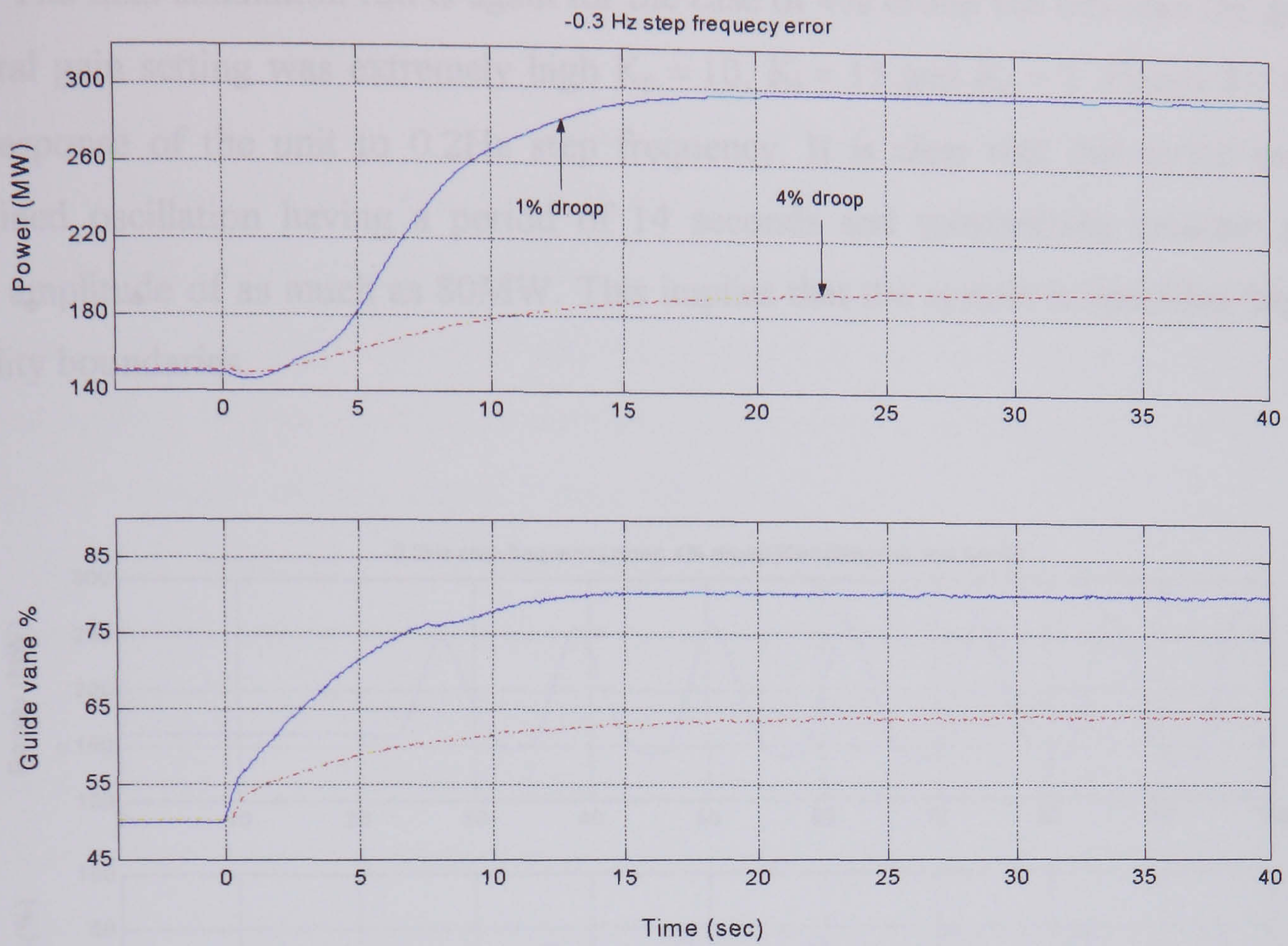
Figure 8-12: HIL simulation response to -0.3Hz step frequency
