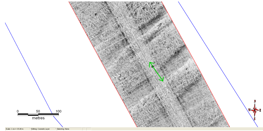
Plate III. In both surveys the environment is characterized by sand ribbons covering coarser substrate. However, as indicated by the arrows the position of the ribbons changed between the 2 surveys.
