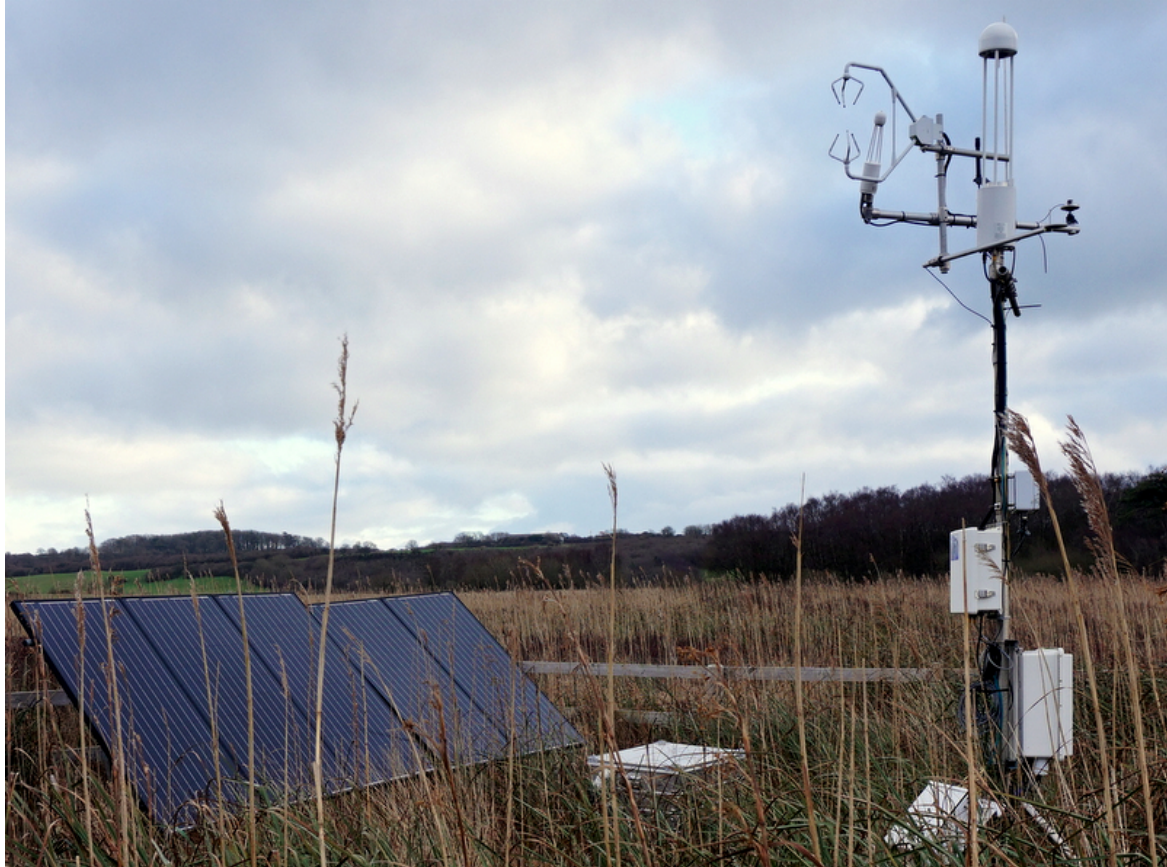
Figure 1.3. A typical system of EC-based measurements at Cors Erddreiniog. Photo by Yingying Xuan on 9 Feb 2016, edited by Yufeng He.
