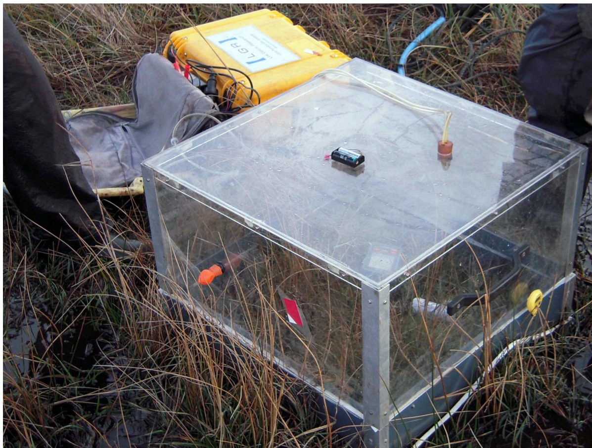
Figure 1.2. An example of chamber-based measurements using a cube at Cors Erddreiniog national nature reserve, Anglesey. Photo by Yufeng He on 17 Dec 2013.
