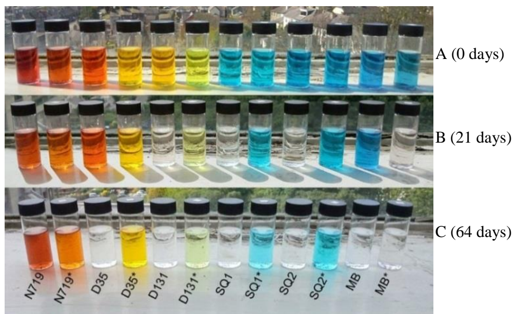
Figure 4.7 Dye solutions of 0.5 mM exposed to sunlight for (Image A) 0 days, (Image B) 21 days, (Image C) 64 days. Dyes marked with an * have an additive of 10 mM TEMP.
