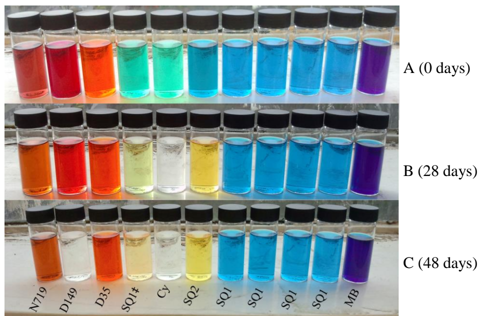
Figure 4.2 Ethanol dye solutions in glass sample vials. Note N719, D149, SQ1‡, Cy and SQ2 were all at a concentration of 0.05 mM the remainder of the dyes had a concentration of 0.5 mM. Note that the solution SQ1‡ was pre-exposed 2 weeks prior to the start of this experiment. The dyes marked Cy and MB represent cyanine and methylene blue dyes. Images show an exposure time of (Image A) 0 days, (Image B) 28 days, (Image C) 48 days.
