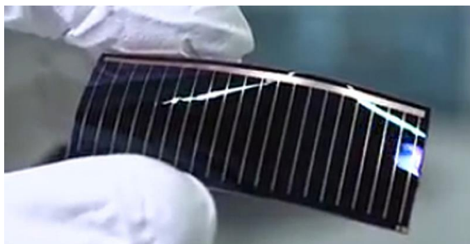
Figure 2.16 Image of a gallium arsenide cell, demonstrating the flexibility of the device without damage. Image taken from literature 135 .
