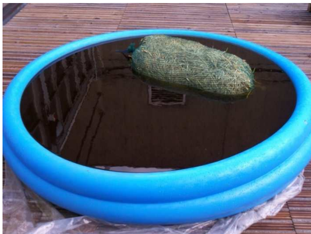
Figure 2.13 – Pond scale 480L mesocosm showing a barley straw boom, which replaced the FCW
