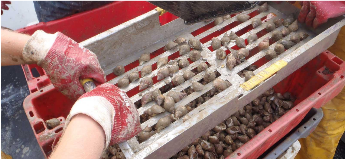
Figure 1.5. A commercial whelk riddle in use, whelks below the Minimum Landing Size (MLS) can be seen collecting in the red container beneath the riddle. Whelks above the MLS are seen caught between and on the riddle bars. ( http://www.kentandessex-ifca.gov.uk/ ).
