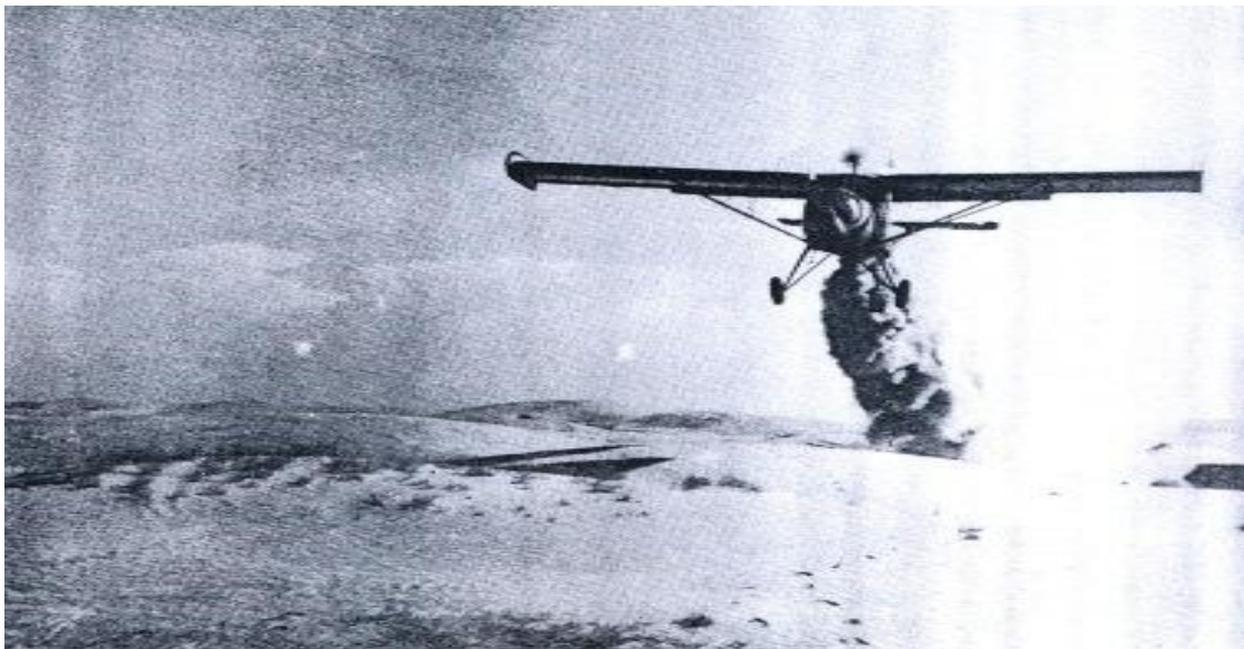
Figure 2.21: Spraying of chemicals from the air in an attempt to sand stabilisation: This figure illustrates an attempt of sand dunes stabilization by spraying of chemicals from a small aircraft, in Al Gawea village in Algarabulli district in 1968 (Khatabi, 1981).
