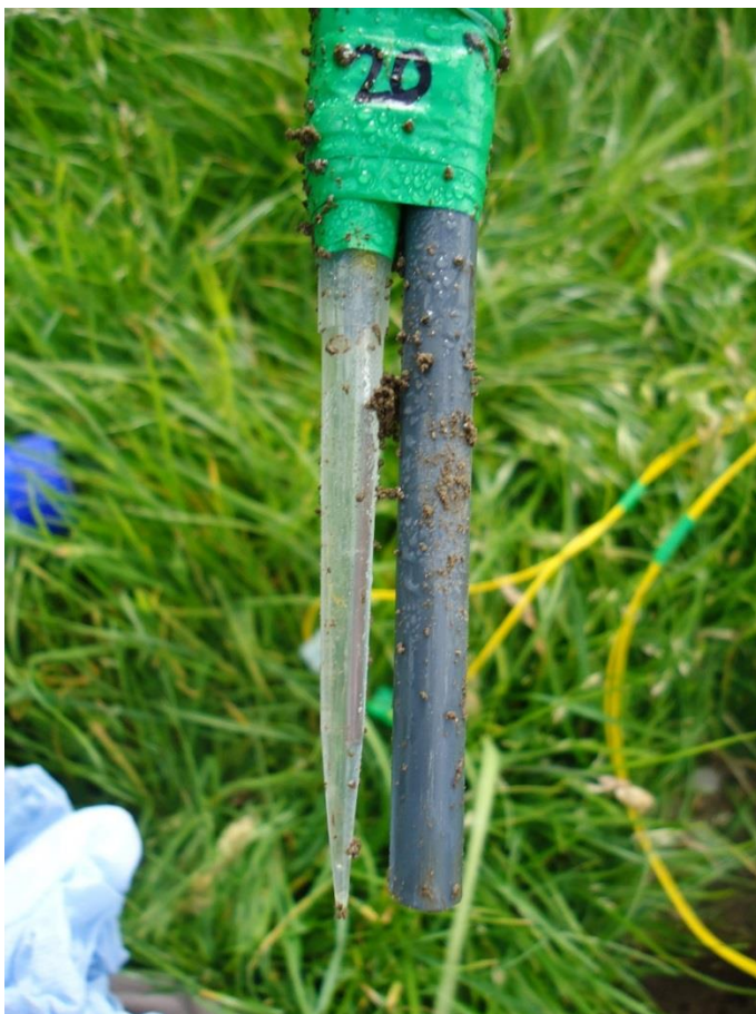
Figure 6. A \text{NO}_3^- ISE removed from the soil following 6 days of continuous, real-time monitoring (Article IV).
