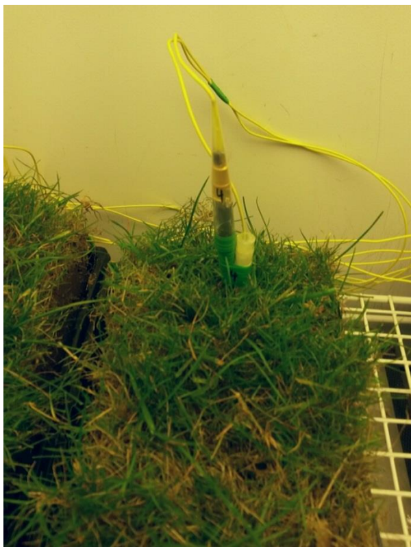
Figure 4. Close up of a \text{NO}_3^- ISE placed in a turf for real-time monitoring (Article IV).
