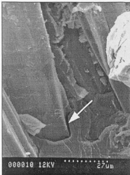
Plate 3.7 Debonding cracks in jute reinforced polyester.
