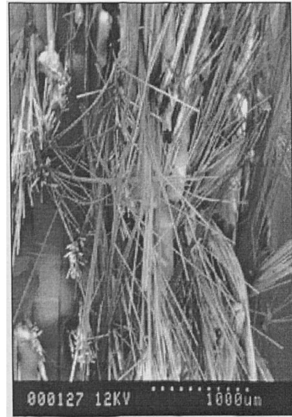
Plate 3.5 Fracture surface of a CSM glass fibre reinforced laminate.
