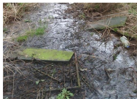
Figure 2.11: Representation of effluent ponding caused by soil clogging and hydraulic failure. Photo was taken during PhD field work.
