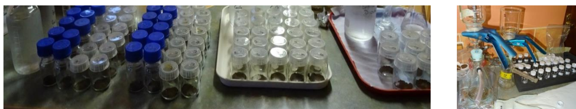
Figure S6.1: Preparation of batch equilibrium experiment (left) and filtration after equilibration (right).
