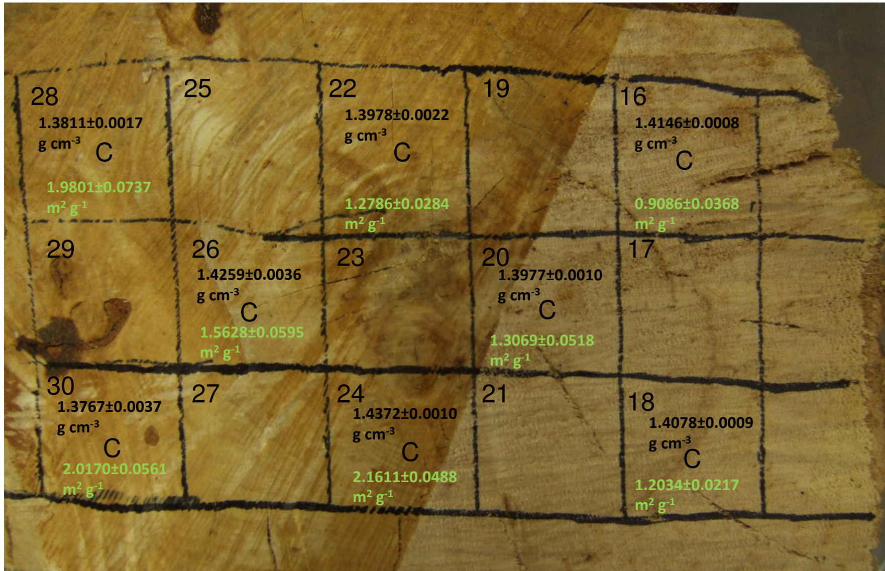
Figure 5.6. Char samples from the second layer of the Malus log (samples 16-30) with the density (black) values and surface area (green) for that sample represented. Scale 1:1.
