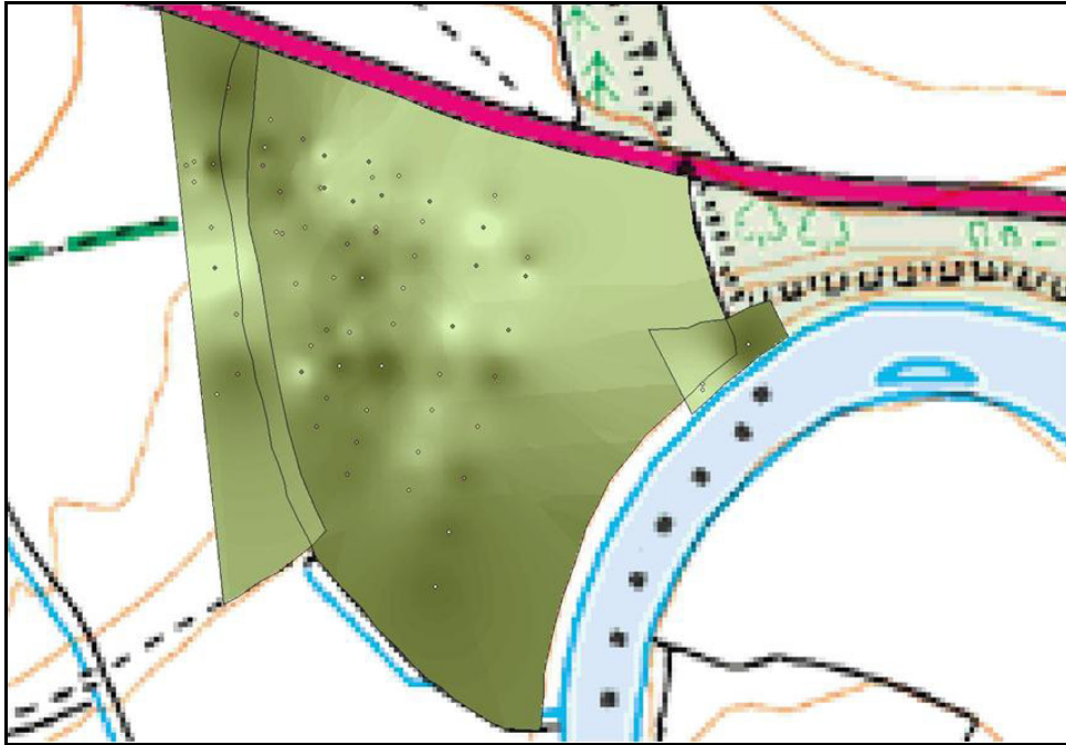
Figure 2.1.3. Site 3 map indicating soil C using data collected (the dots on the map) and interpolated to create a continuous surface using the inverse distance weighted (IDW) method on ArcMap (ArcGIS version 9.3.1 ESRI, 2009). Areas in a darker shade indicate higher levels of carbon. © Crown copyright / database right 2010. An Ordnance Survey / EDINA supplied service.
