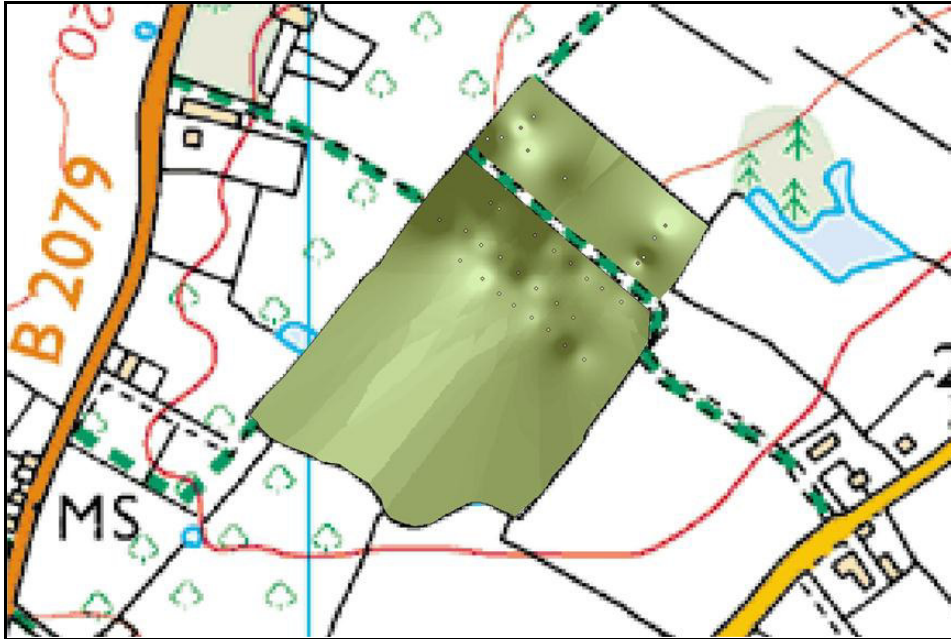
Figure 2.1.5. Site 5 map indicating soil C using data collected (the dots on the map) and interpolated to create a continuous surface using the inverse distance weighted (IDW) method on ArcMap (ArcGIS version 9.3.1 ESRI, 2009). Areas in a darker shade indicate higher levels of carbon. © Crown copyright / database right 2010. An Ordnance Survey / EDINA supplied service.
