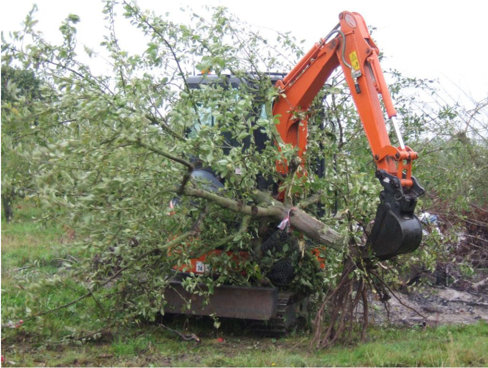
Figure 3.2. Orchard tree being grubbed-out, where the whole tree including roots and stump are removed from the ground.
