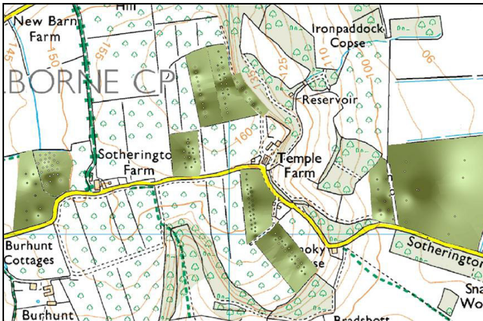
Figure 2.1.4. Site 4 map indicating soil C using data collected (the dots on the map) and interpolated to create a continuous surface using the inverse distance weighted (IDW) method on ArcMap (ArcGIS version 9.3.1 ESRI, 2009). Areas in a darker shade indicate higher levels of carbon. © Crown copyright / database right 2010. An Ordnance Survey / EDINA supplied service.
