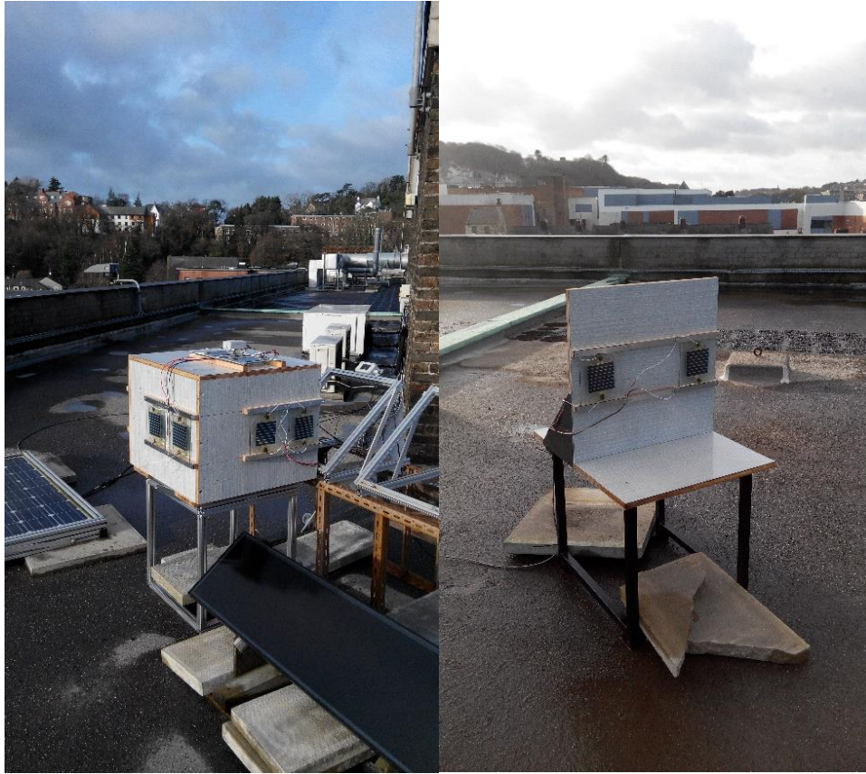
Figure 5.9 – Outdoor Organic BIPV test rigs after their installation. East, South, West and Horizontal/Flat modules mounted on cuboid shape industrial building prototype (left), North facing modules mounted on a separate panel (right).
