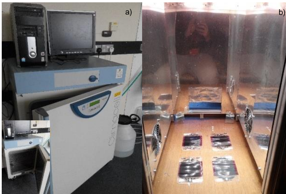
Figure 3.11 – a) Climacell 111 - Comfort environmental chamber capable of keeping a constant temperature from 0^{\circ}\text{C} to 100^{\circ}\text{C} and relative humidity up to 100%. b) halogen solar simulator used for the execution of this experiment
