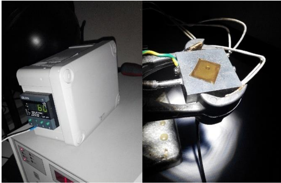
Figure 3.6 – Indoor test setup at Bangor University. Newport standard AM1.5G light source and heated platform keeping a constant ambient temperature.
