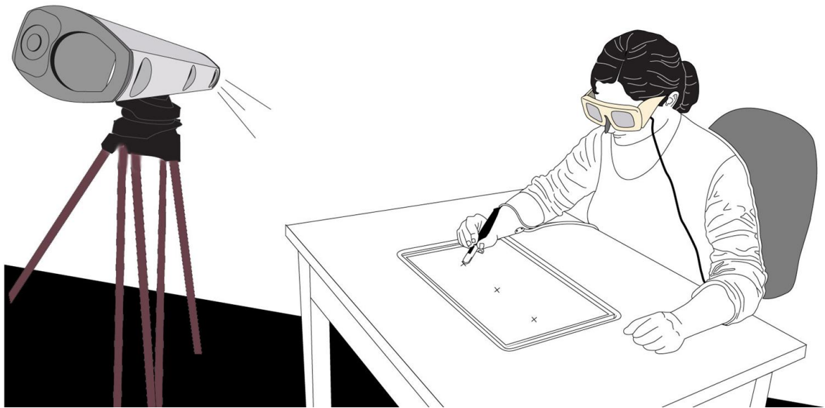
Figure 5 schematic representation of the experiment set-up .the aiming task was performed with a stylus to target displayed on a computer monitor that was mounted facing upwards in a cavity cut out from a table top. Movements were performed in the right to left direction.
