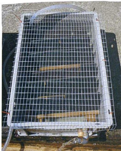
Figure 2 a-c. a) Diagrams showing the procedure used for the biofilming of experimental surfaces: slate tiles and assay slates and glass microscope slides. b) Tanks with running seawater used for biofilming of slates outside laboratory; two tanks were fed constantly with running seawater, the other (middle tank) was drained for 3-4 hours daily. c) slates held in grooved wooden racks within tank. Seawater (gravity fed from the laboratory system at 2 l/min) was fed into the bottom of the tank at one end and drained from the other end.
