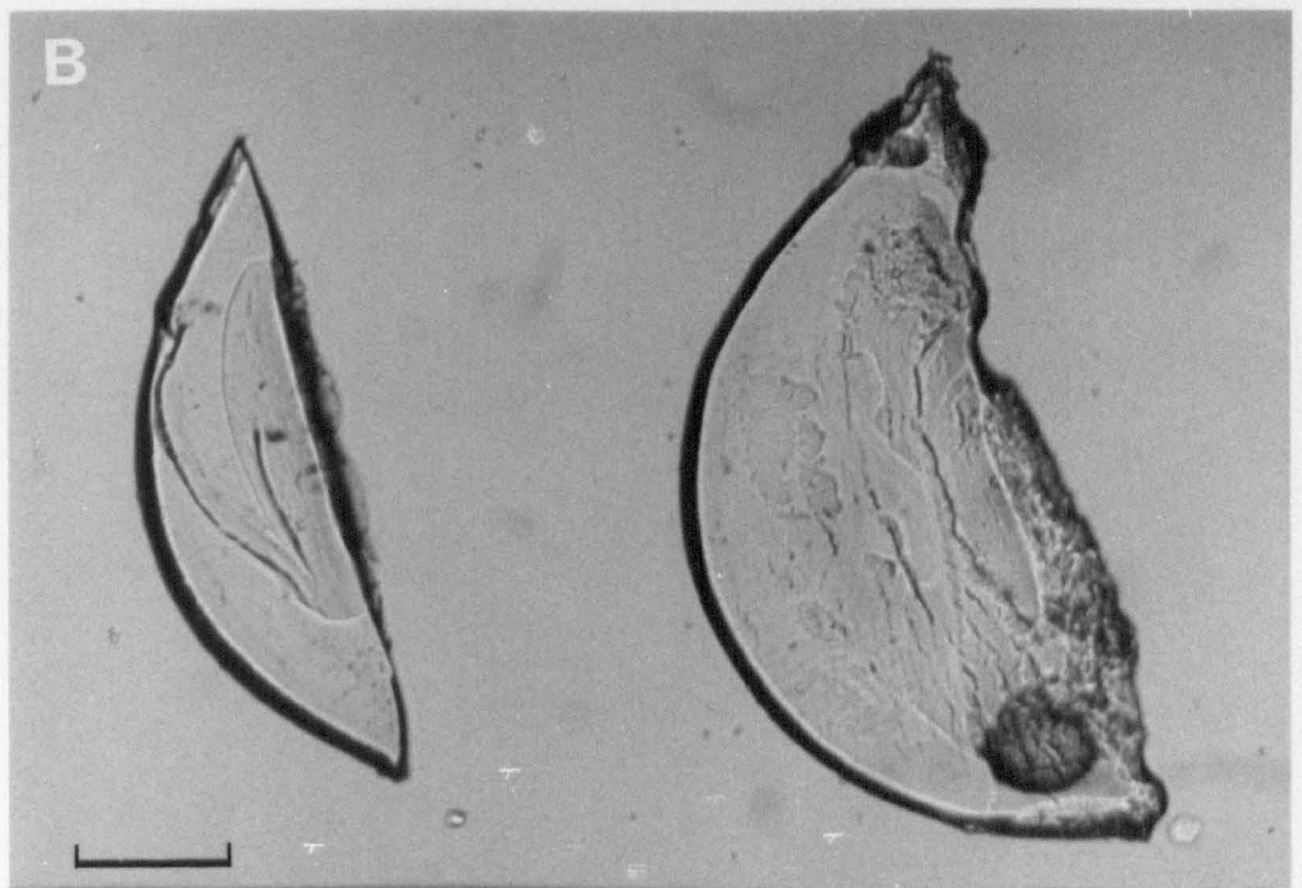
Figure 8: A; hand cut sections of Pollicipes pollicipes cement viewed with transmitted light. The cement is translucent to transmitted light but zonation is obvious. The outer zone (oz) is more translucent than the inner zone (iz) probably due to less light refraction from absorbed water. B; the same sections after heat treatment (see text) resulting in an homogeneous, fully translucent appearance. Scale bar is 200 \mu\text{m} .
