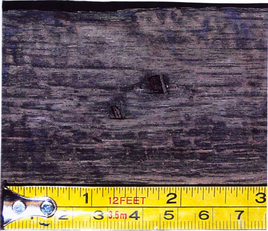
Fig.1.7a- Logboat clenched wrought iron nails.
