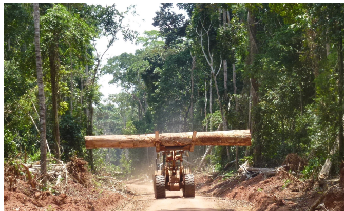
Figure 1 – Wheeled loader with log fork on a logging road in Republic of Congo
