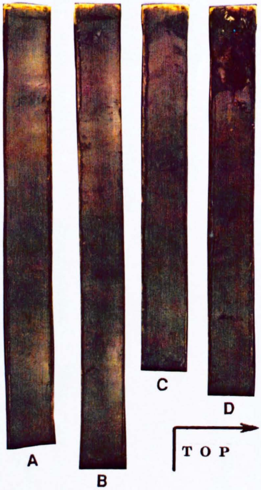
Plate II.1. BGS Borehole and vibrocores from the Inner Silver Pit, southern North Sea.
