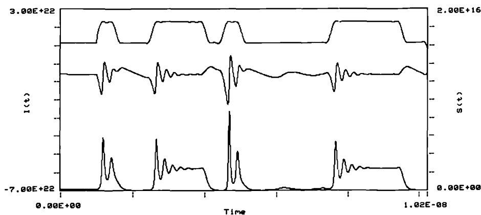
Fig.2.4 DFB Laser Current, Instantaneous Wavelength and Optical Power (top to bottom)
