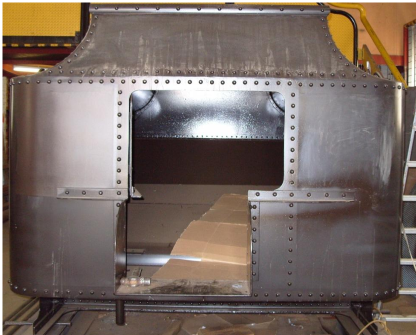
7.1.5. New Tender for the Welsh Highland Railway Locomotive NGG16 Class Garratt number 87.
