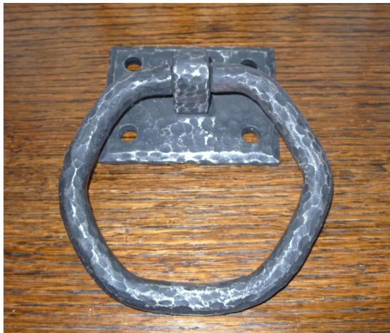
Photo 5.11. Replica coffin handle hand made from wrought iron, antique hammered and polished by Mr Meurig Williams for Mr Graham Lay. Photographed by Pam Smith 2010.
