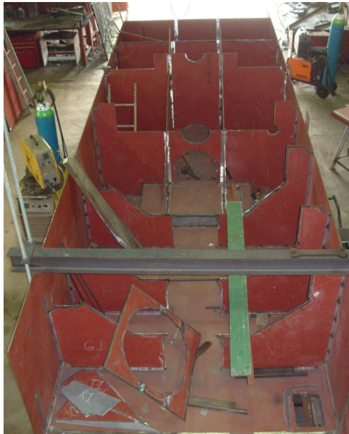
Photo 6.1. Tender for NG15 Number 134 constructed at Brunswick Ironworks June 2011. Photographed by Pam Smith.
