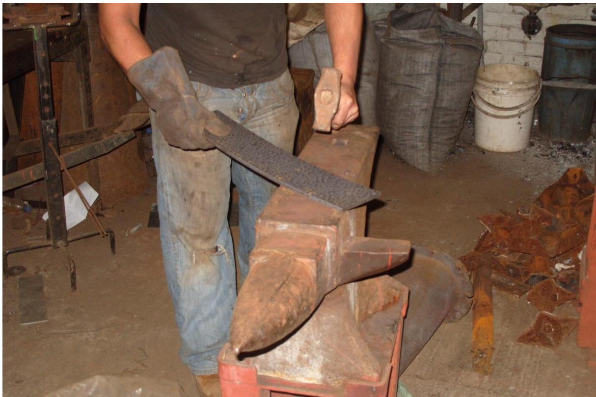
Photo 3.65. The bands for the coffin were antique hammered by the craftsmen at the Brunswick Ironworks, Photographed by Pam Smith 2010.
