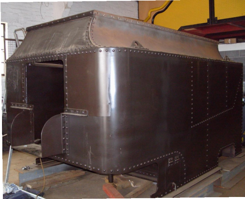
7.8. Welded and riveted tender for narrow gauge locomotive.
