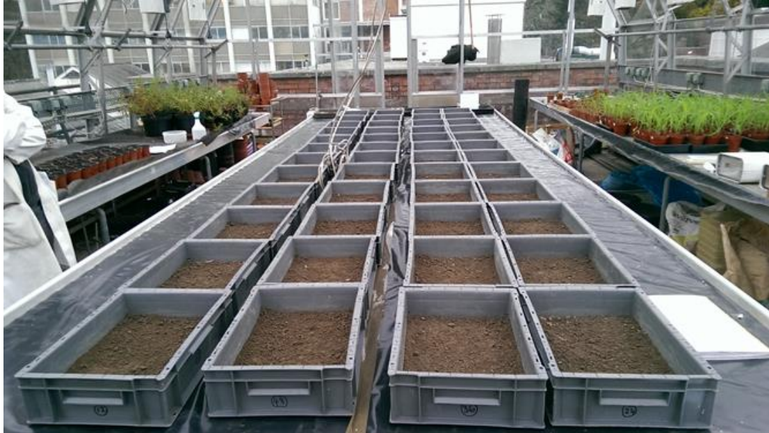
Figure 1 Eutric Cambisol mesocosms maintained at 50% and 70% WFPS.
