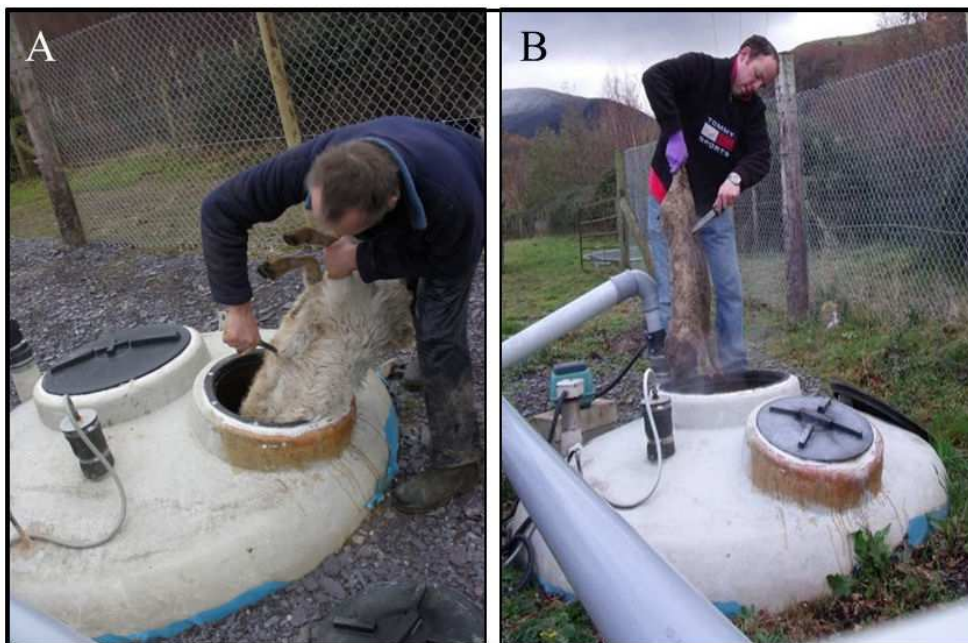
Figure 3: An incision is made into the abdomen of both sheep (A) and pig (B) carcasses before inputting into the vessels.
