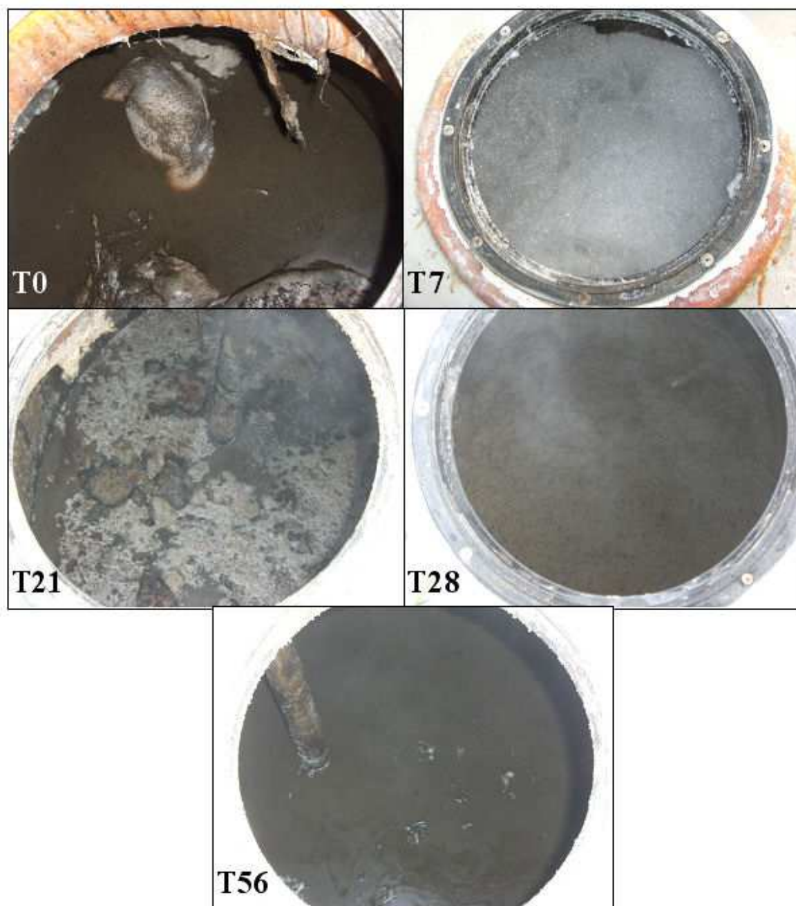
Figure 1: The sequential degradation of pig carcasses over a 56 day bioreduction trial. T = time after carcass addition in days.
