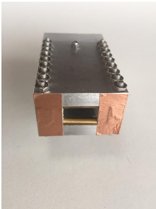
Figure 74 Front view showing aperture with foil reflectors fitted over PTFE side blocks
