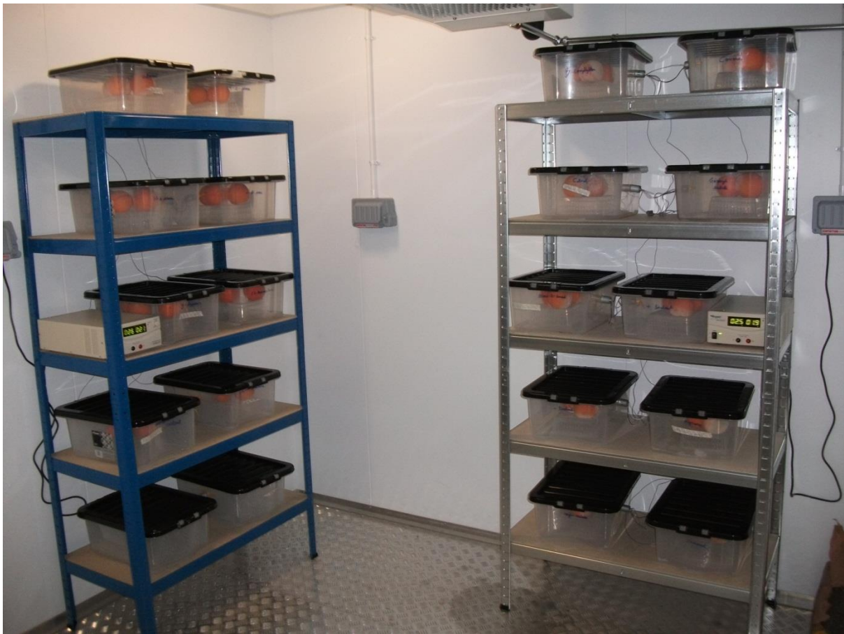
Figure 2.06: Containers set up in a (dark) controlled temperature room. Different relative humidities (RH) were maintained in each container using saturated salt solutions. Air circulation in each container was achieved by using motorised fans linked to a power supply on each set of shelves.
