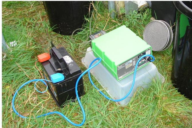
Figure 8.4. Peristaltic pump used for manure slurry addition in Run 2.
