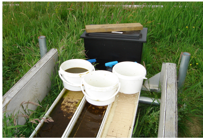
Figure 8.3. Buckets used for manure slurry addition in Run 1.
