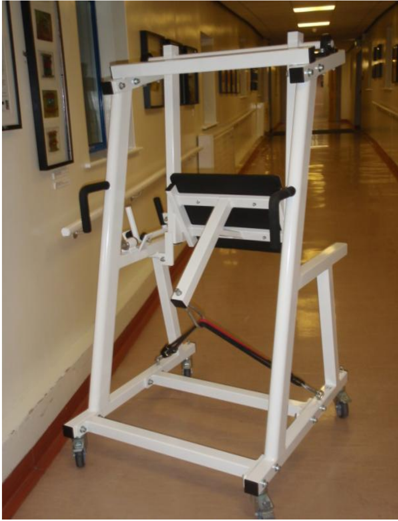
Figure 5.1. Novel resistance exercise equipment (Fitness Systems, Bolton, UK) designed equipment designed to fit to the end of a dialysis chair (Stephen H Anatomical New, Gardhen Bilance, Pomigliano d'Arco, Italy). The leg press equipment utilised a series of resistance bands providing a maximum resistance equivalent to 200 kg.
