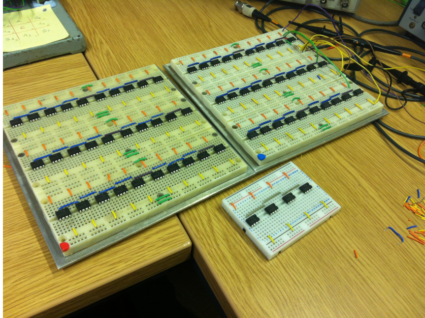
Figure 4.25: All 64 op amps configured to be Comparators
