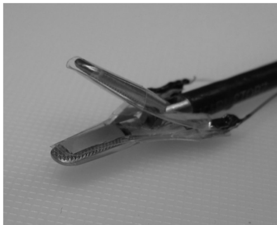
Figure 2.17: A robotic grasper with a thin piece of piezoelectric material overlaid on the bottom to sense contact with tissue [71]
