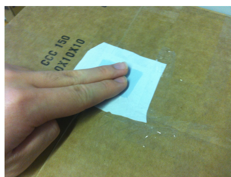
(b) The cutout on top of the box. The polythene material is actuated by the focal point emitted from the hemispherical array situated inside the hollow box.
