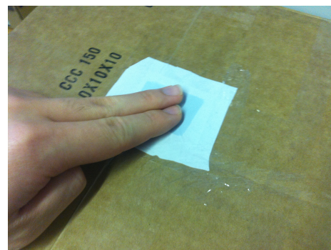
(b) The cutout on top of the box. The polythene material is actuated by the focal point emitted from the hemispherical array situated inside the hollow box.
