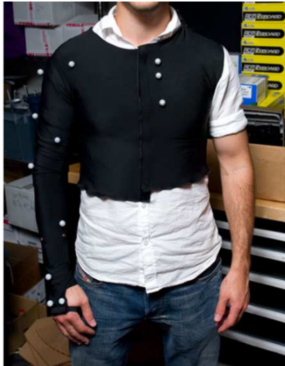
Figure 2.16: A wearable vest with hidden vibration motors embedded at selected joint positions. The white markers aid in optical tracking of the limb [66]
