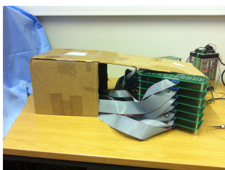
(a) A hollow box was placed above the array to provide a solid interface for users to interact with.
