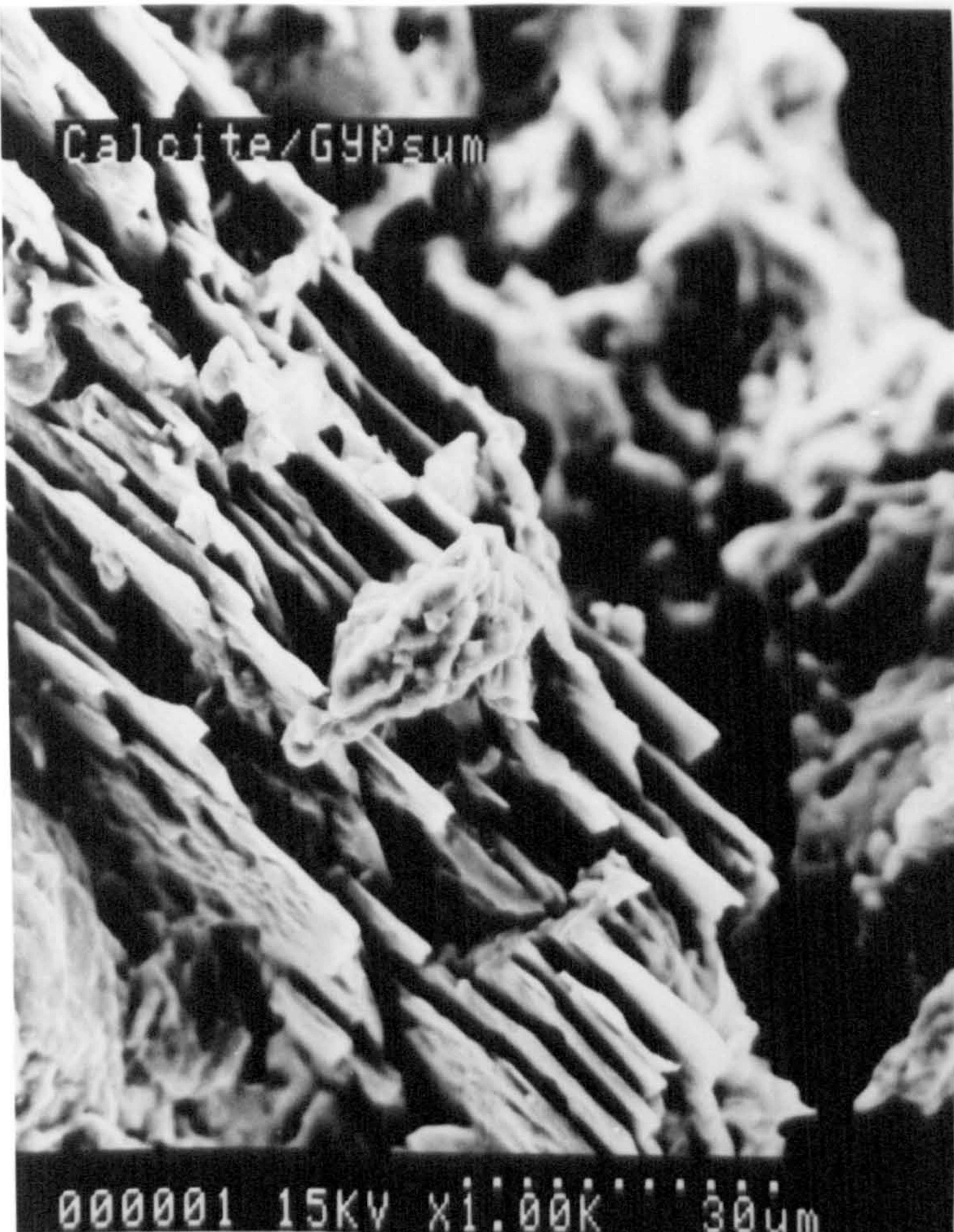
A broken formation of gypsum crystals with a calcite particle wedged between layers.
