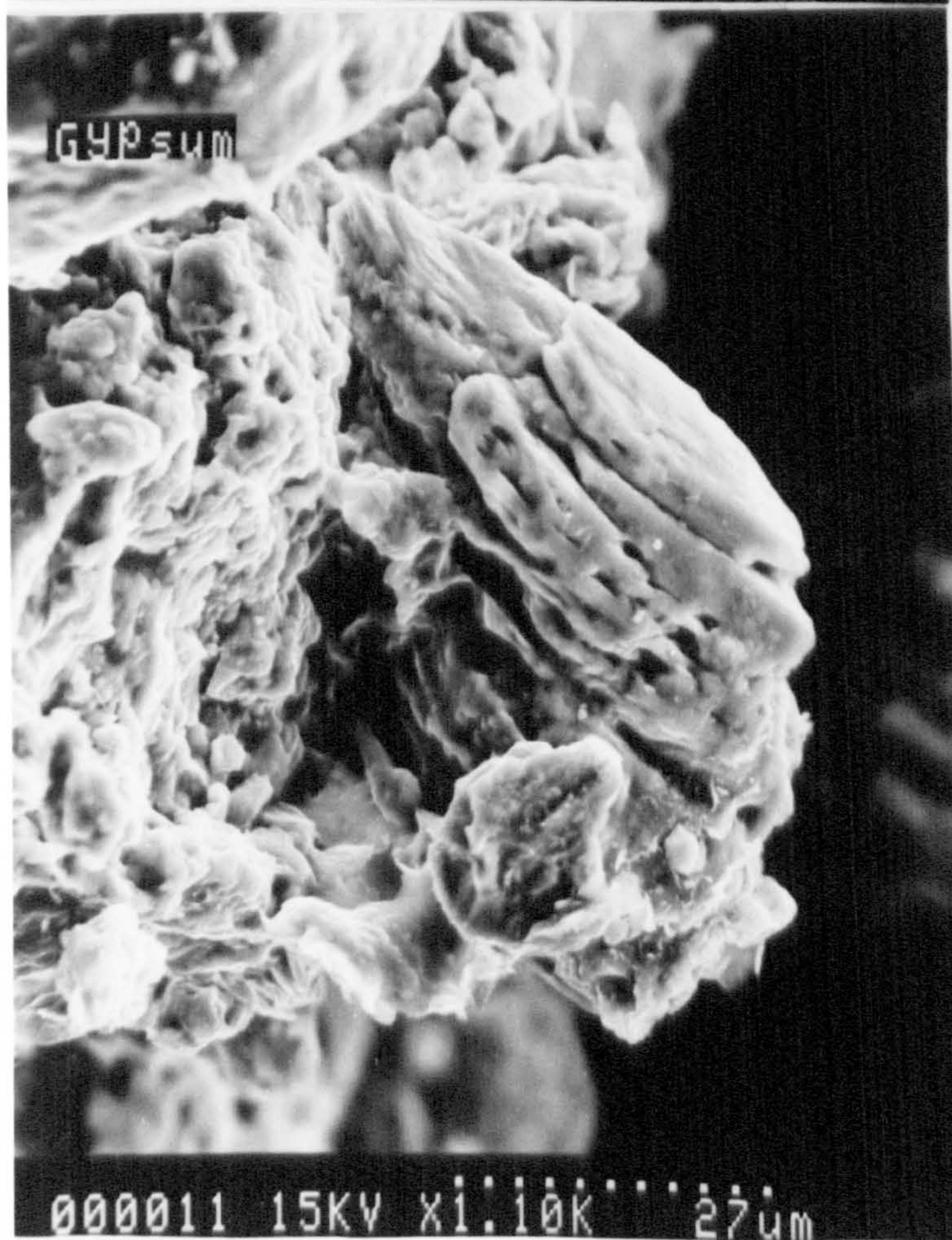
Gypsum ( \text{CaSO}_4 \cdot 2\text{H}_2\text{O} ); the poor crystallinity of particles may indicate recent deposition.
