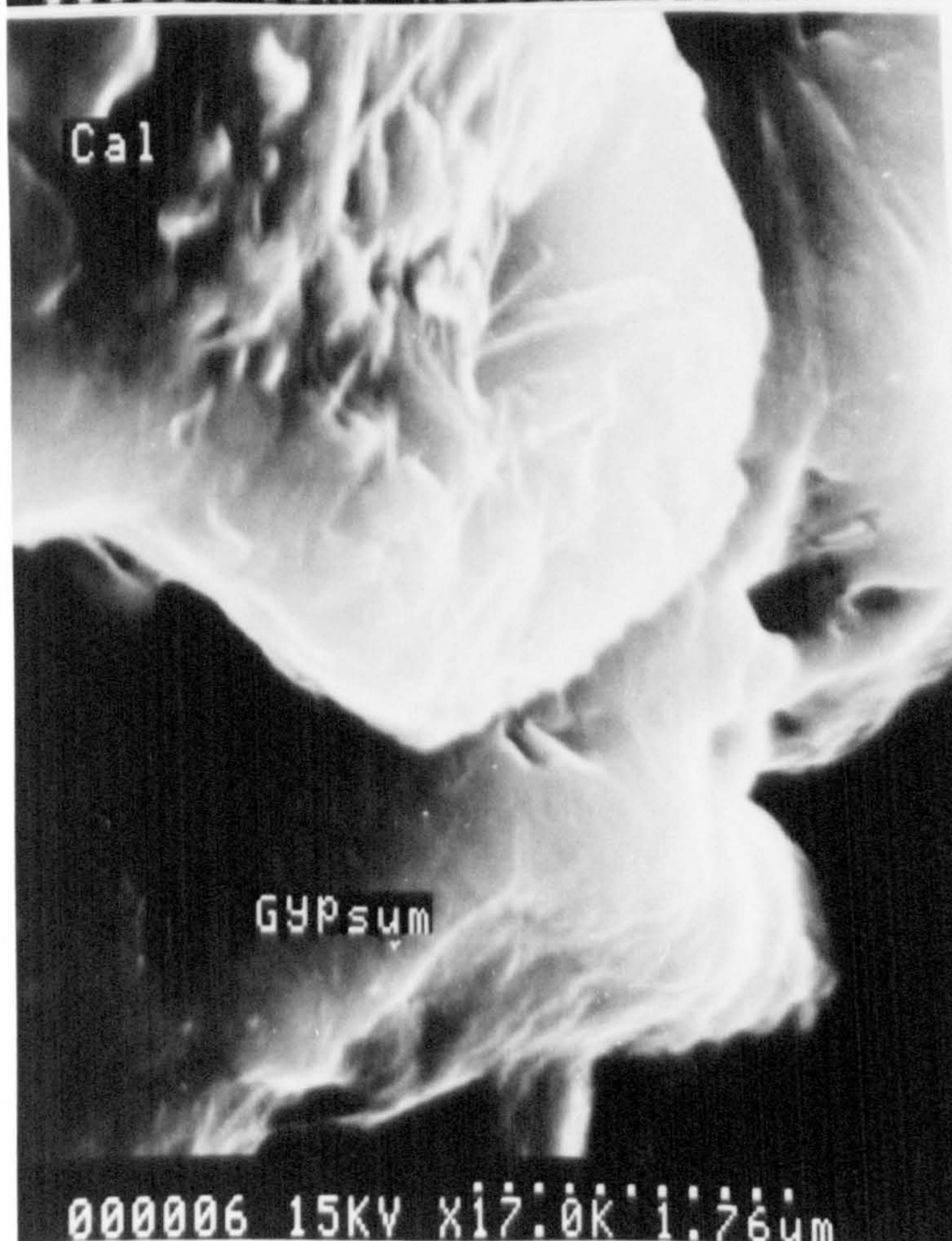
At higher magnification, a degree of reduction in calcite exposed surface area is shown.
