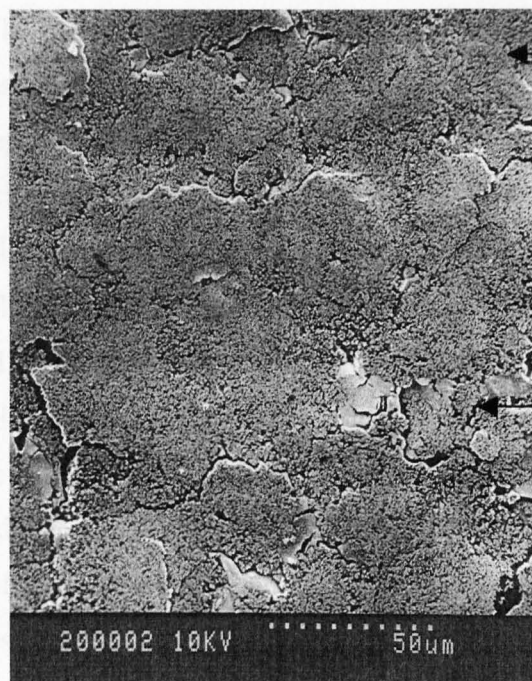
Figure 30c SEM image of compressed rhodium after galvanostatic deposition for 14 hours ( \times 600 )
