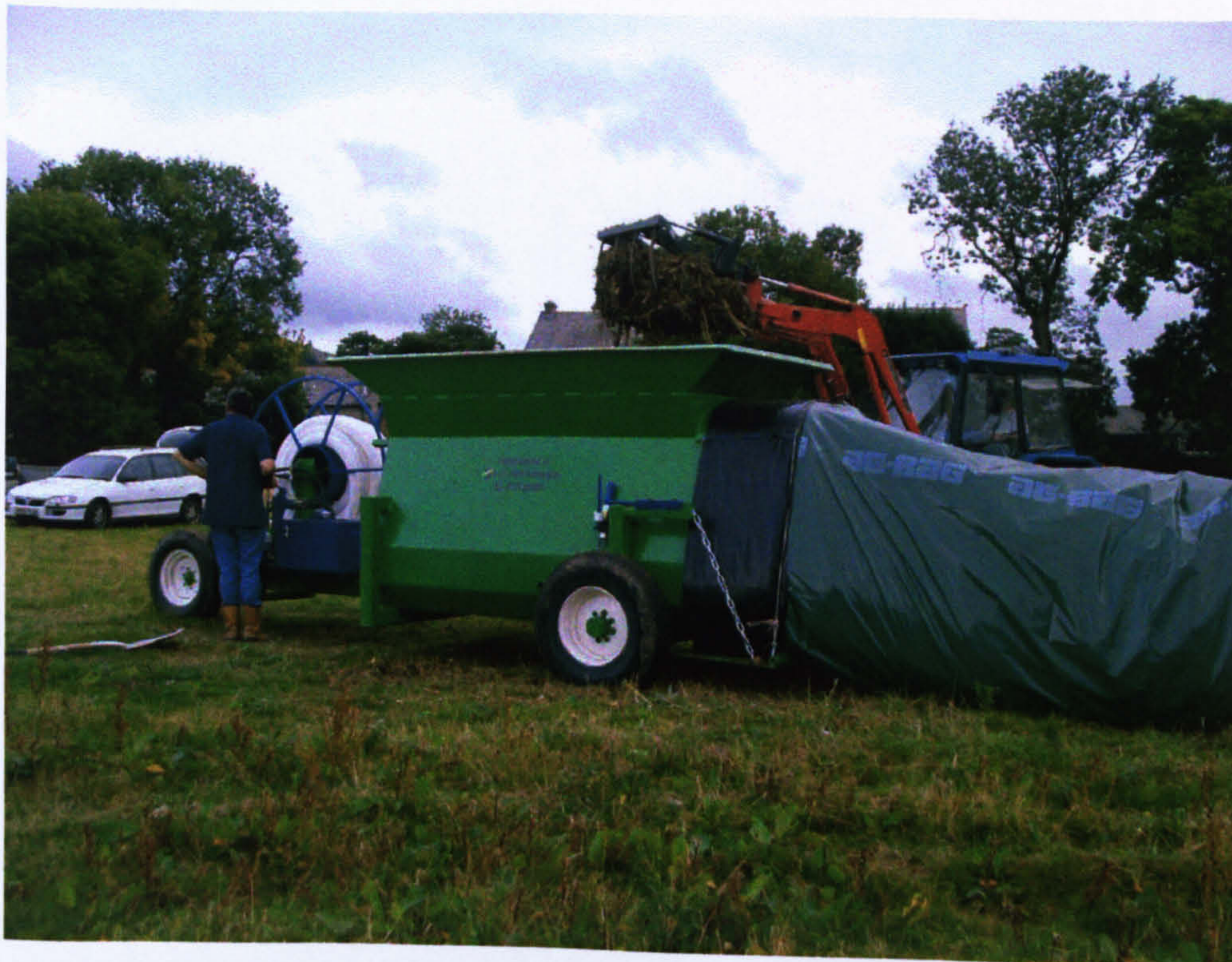
Figure 3.2 Filling the CT5 ® with green waste
