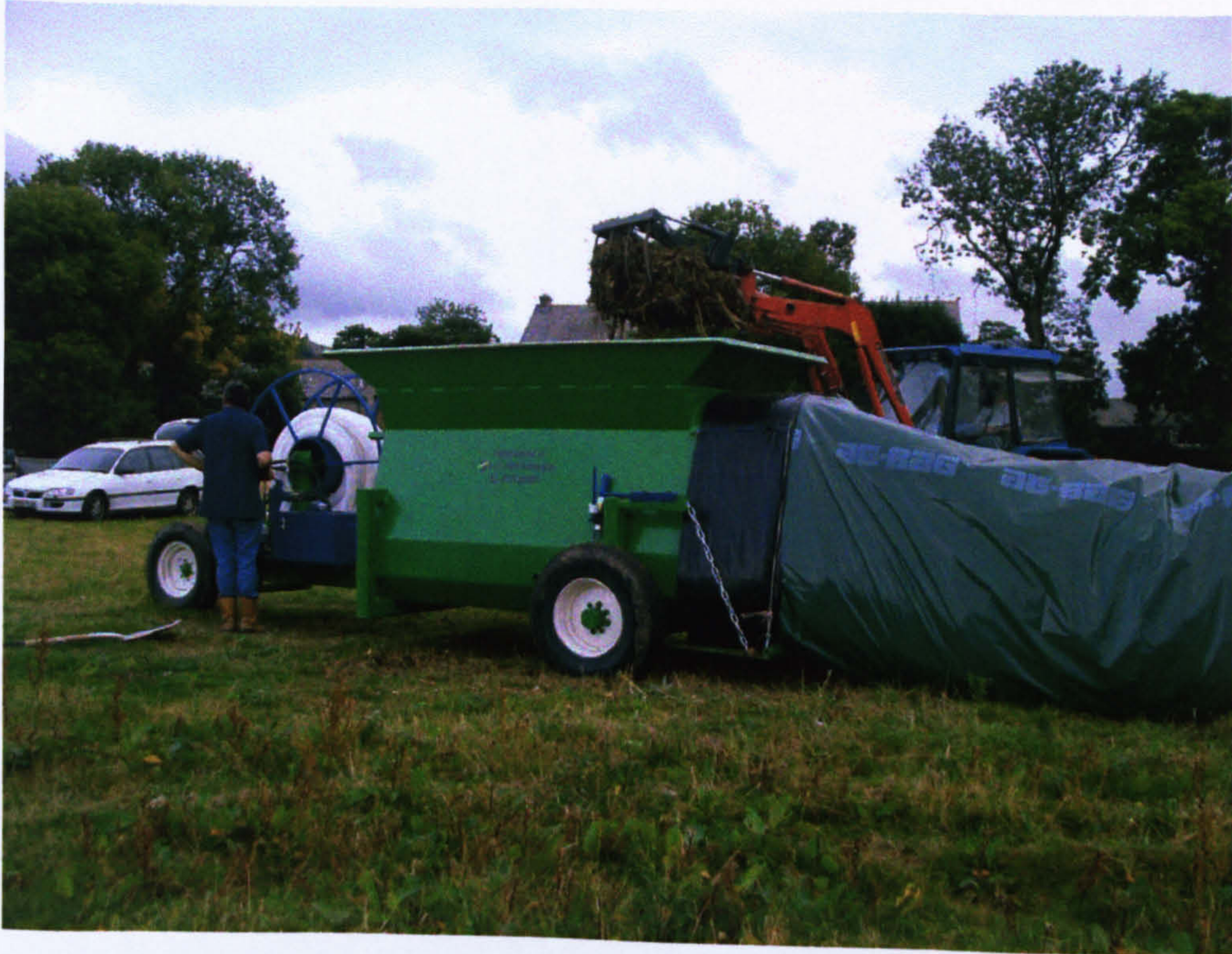
Figure 3.2 Filling the CT5 ® with green waste
