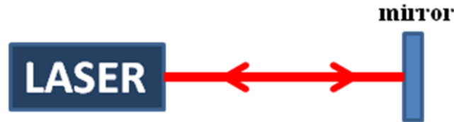
Figure 2.2 Schematic setup of the SL subject to optical feedback
