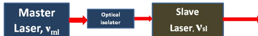
Figure 2.1 Schematic setup of the master-slave laser configuration Optical isolator is used for unidirectional coupling.
