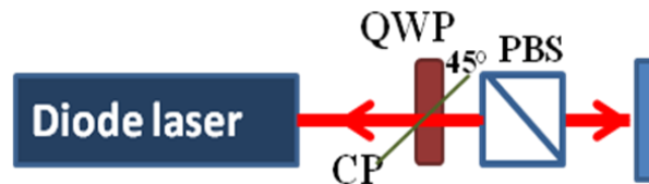
Figure 4.2: circularly polarised optical feedback.
