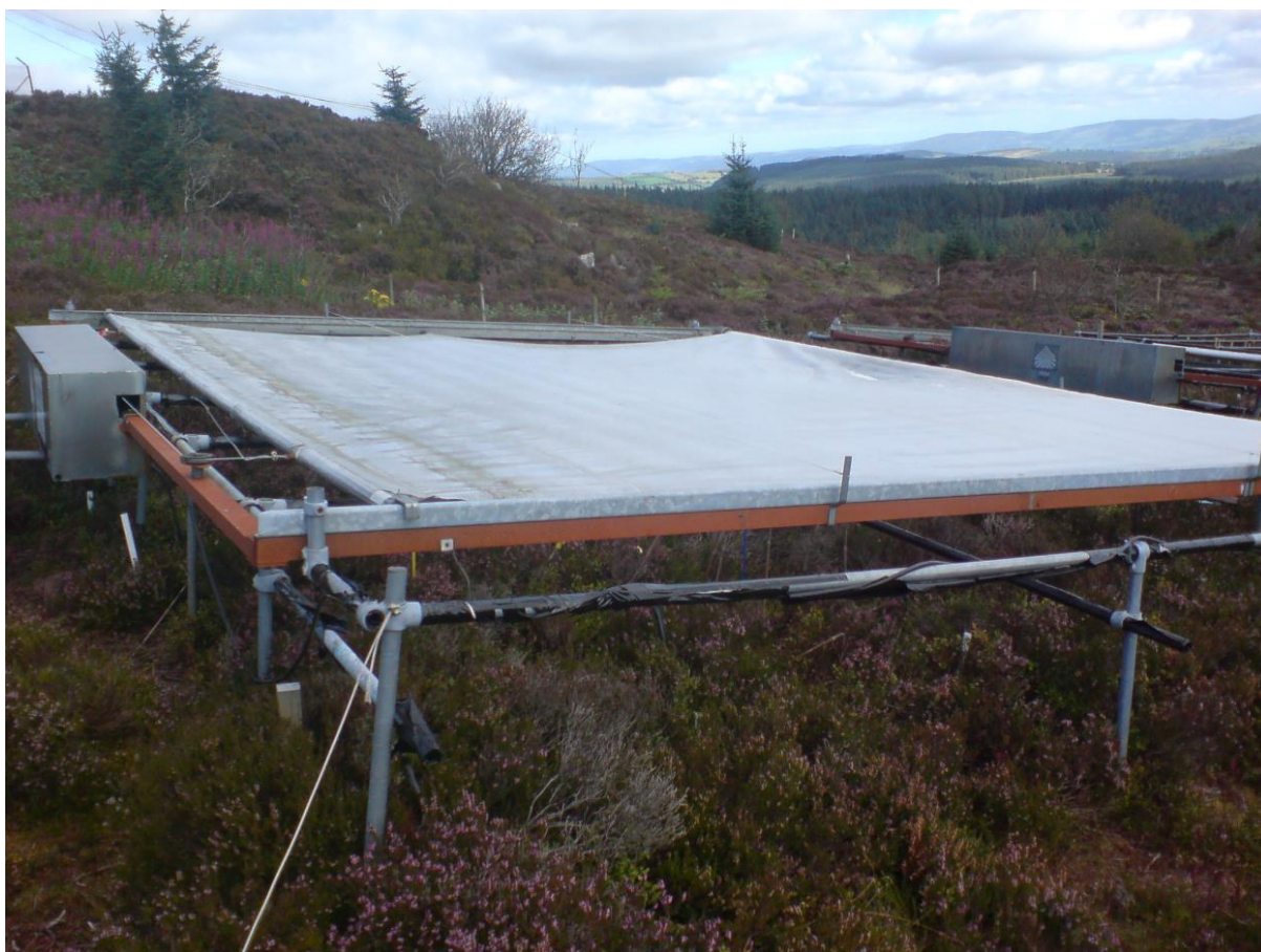
Figure 3.2.1 Photograph of a drought plot with roof extended over the plot.
