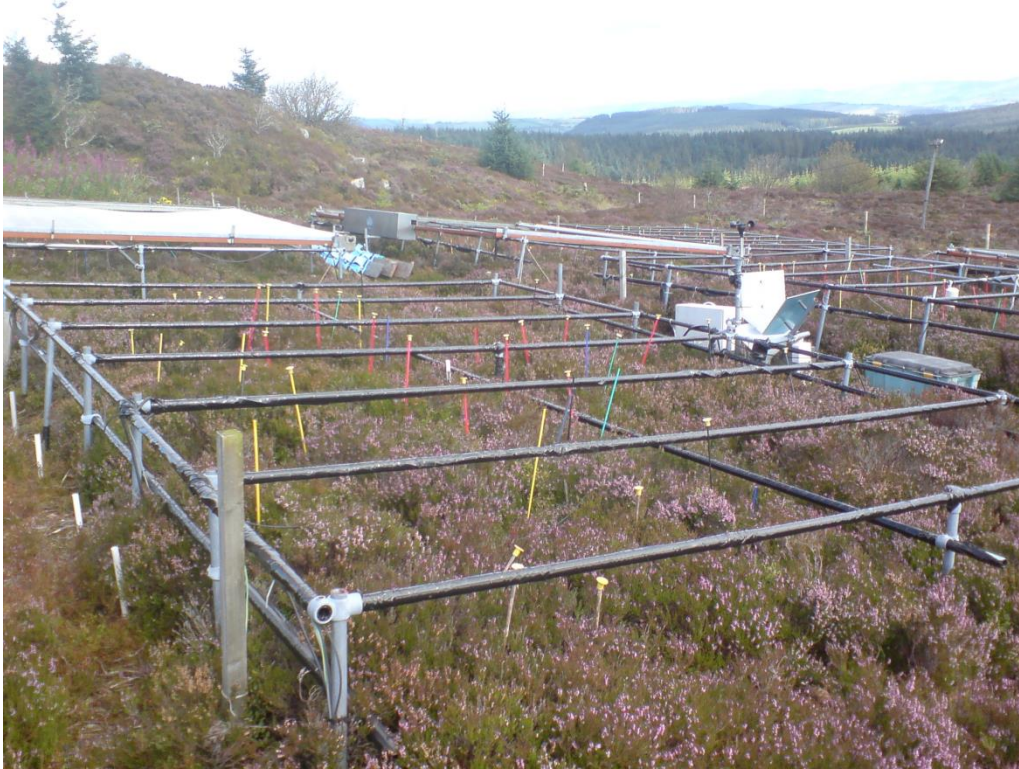
Figure 2.2.1 Photograph showing general plot layout with control plot in the foreground, and an extended roof shown for demonstration over a plot.
