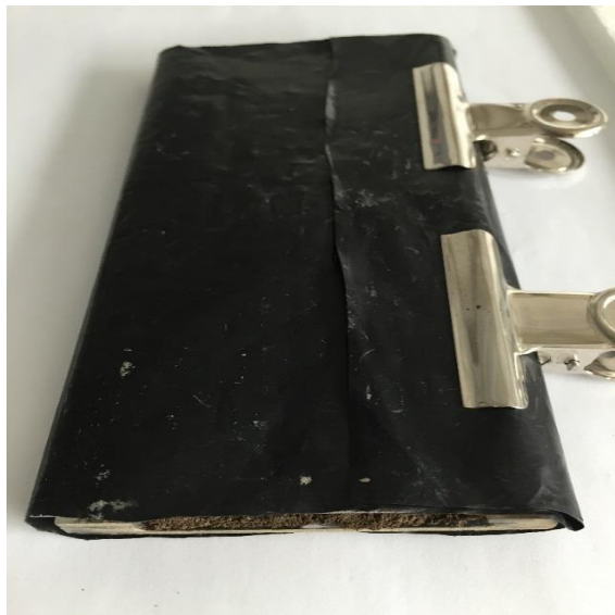
Plate 2.1 Microcosm (see Figures 2.1 and 2) filled with 50 g of soil and covered with black plastic.
