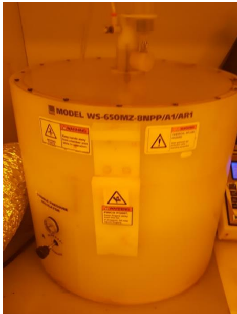
Figure 3.6 Spin coater (Model WS-650MZ-8Npp/A1/AR1).
