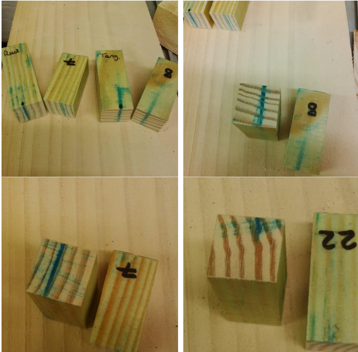
Figure 3. (a) Cross section of southern yellow pine, made just below the laser incision to reveal longitudinal flow from the incision. (b) For a radial incision in SYP, the cascade pattern of impregnation in earlywood and latewood, revealing radial transport of fluid in addition to longitudinal flow. (c) Prominent radial transport of fluid away from laser incision region in a tangentially incised sample of SYP. (d) Radial flow of fluid away from incision line in an incision into a half-radial face of SYP.
