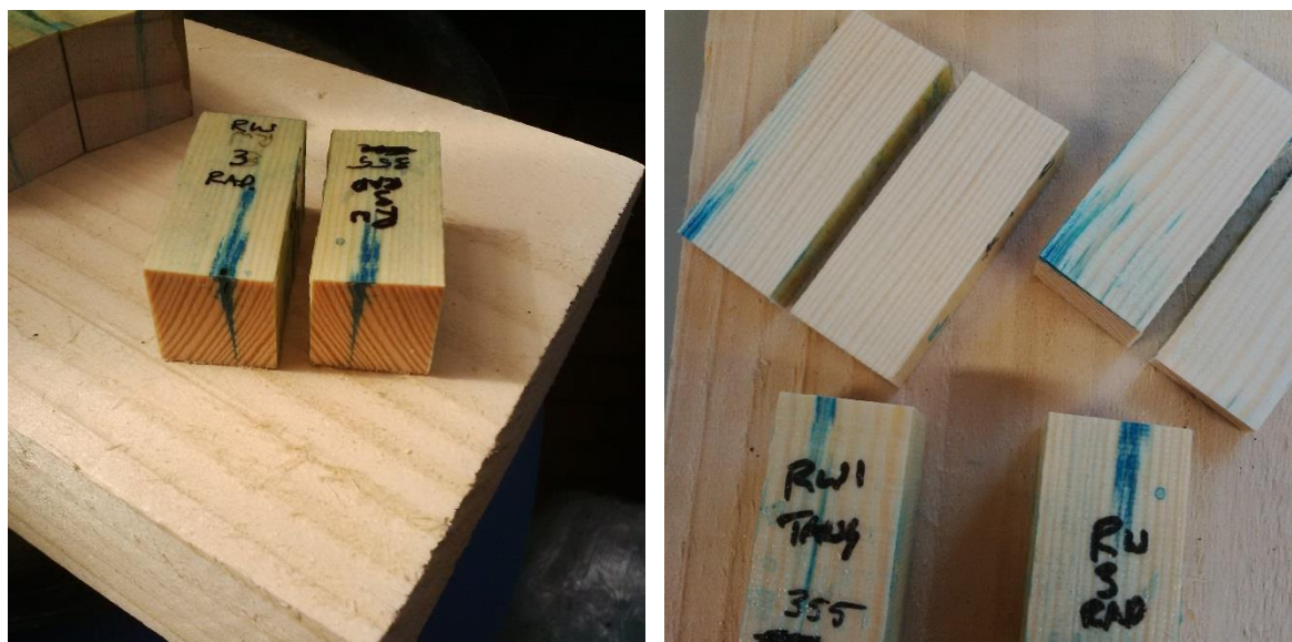
Figure 2. (a) Longitudinal flow is preferential in the latewood of redwood heartwood, with only minor radial flow away from the incision line (incised in the half radial face). (b) Longitudinal flow is preferentially located in latewood of redwood samples, whether incised into tangential (left) or radial (right) face. There was also evidence of longer distance flow within the resin canal system.
