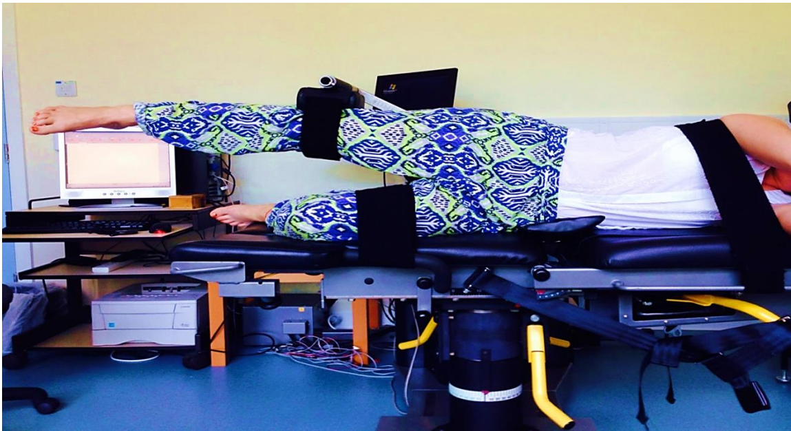
Figure 1: Participant from study 1 on HUMAC dynamometer's table connected with the dynamometer arm at 15°
