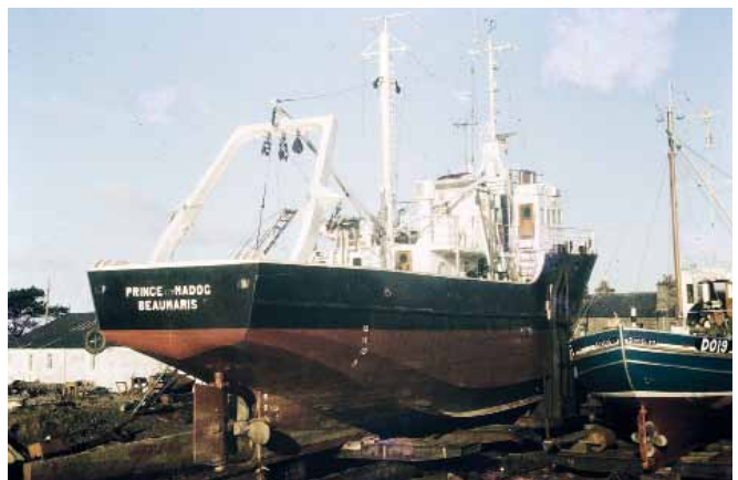
▲ Prince Madog (1968) out of the water, showing the three-blade variable pitch propeller. The stern was modified to be vertical after the hull launch, to aid in handling of scientific equipment from the stern bulwark. IVOR REES
