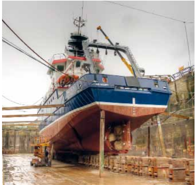
▲ The current Prince Madog in dry dock, showing the stern and ducted variable pitch four-blade propeller. BEN POWELL
