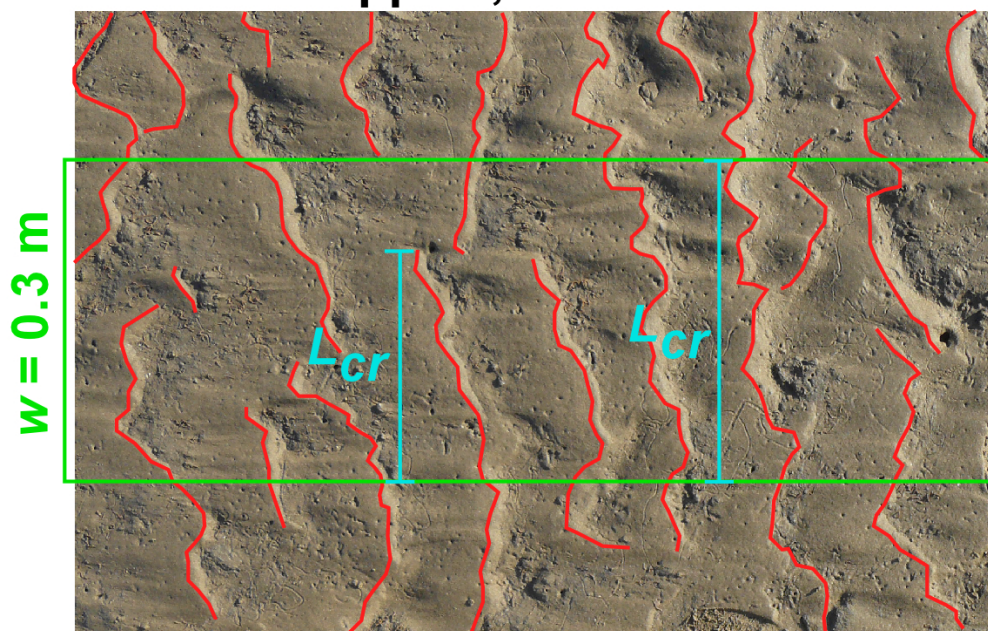
Fig. A1. Summary of the methodology used to calculate ripple planform indices. A 0.3-m wide window was placed in the centre of the picture (in green), before tracing the ripple crestlines within this window (in red). Thereafter, the shortest distance, L_{cr} , between the start and end of each crestline was measured (in blue) and divided by the width of the window to derive the ripple planform index as measure of ripple three-dimensionality. Finally, the average value of I was calculated for each bed.
