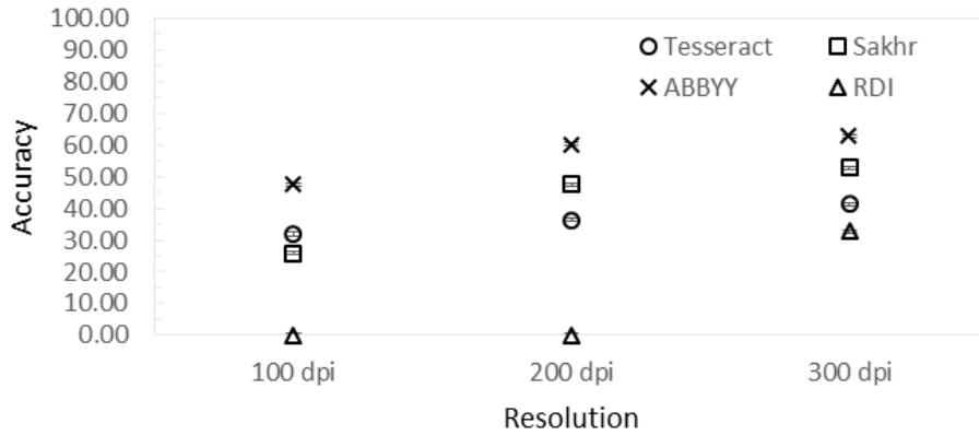
Figure 3.7. Overall accuracy vs. resolution results from the OCR system evaluation
