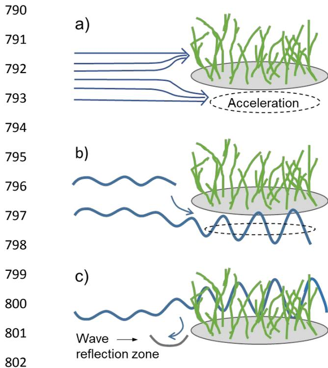
803 Fig 6. Interactions of current flow and waves on erosion around vegetation patches. (a) Diversion of
