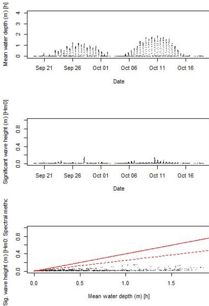
Fig S3. Mean water depths and significant wave heights measured at the three sites (a) Exposed, (b) Moderate and (c) Sheltered over the observation period (September-October 2018).
