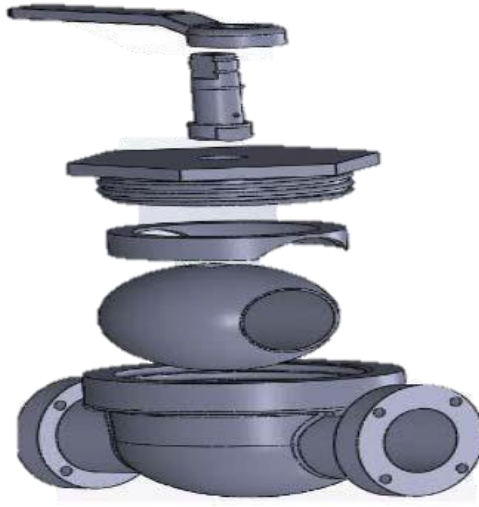
Figure 1.13 DFMA of flow control valve top entry design with 6 components
