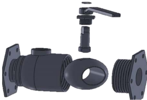
Figure 1.10 Existing flow control valve side entry design with 18 components.
