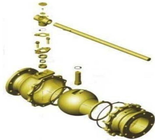
Figure 1.10 Existing flow control valve side entry design with 18 components.
