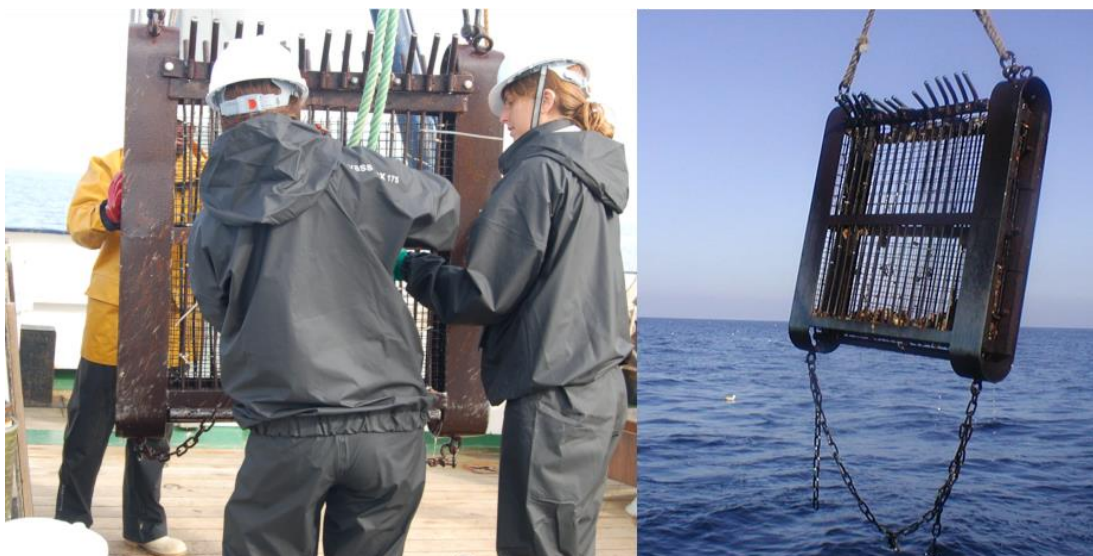
Figure 2.2 Deployment of the Arctica dredge.
