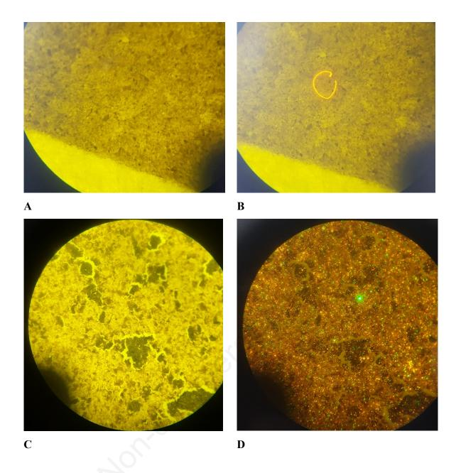
Fig. 1. A section of filter paper looked at through x40 magnification for microplastic identification. a,c) Photographed using only standard, visible light; b,d) photographed using a fluorescence lighting system.
