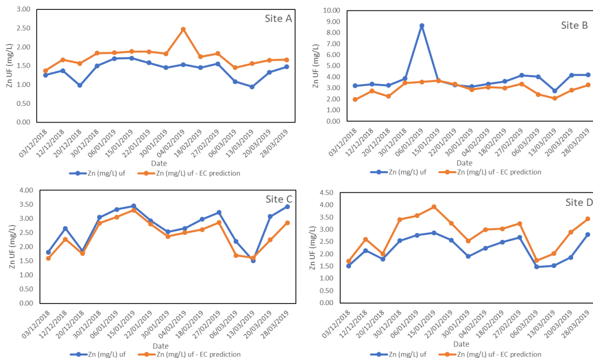
Figure 8.24. Zinc concentration and predicted Zn concentration relationship at Parc sites based on EC data at sites A, B, C and D 27.11.18-28.03.19.
