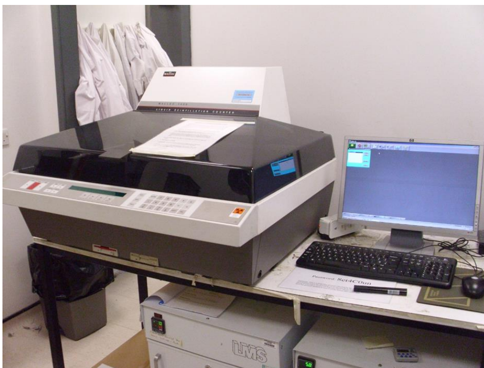
Plate 2: Wallace 1409 liquid scintillation counter located in the counting room and utilised for all ^{14}\text{C} analysis of vegetative, soil sand and liquid samples (Wallac EGandG, Milton Keynes, UK).
