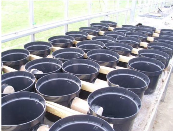
Plate 13: pots were then stapled together with wooded supporting struts to prevent mycorrhizal hyphal from being damaged in transit during the experiment
