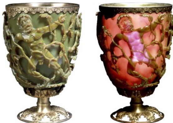
FIGURE 1.3: Images of Lycurgus cup showing the difference between transmitted and reflect light through the glass.
