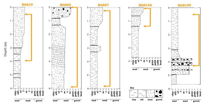
Fig. 3. Lithostratigraphic logs for vibrocores BGS19, BGS65, BGS87, BGS166 and BGS199. The horizontal lines on the logs indicate: gaps in the core record (grey), gradational contacts (black dashed), and abrupt contacts (solid black). The orange arrows indicate the dated extents of the cores.
